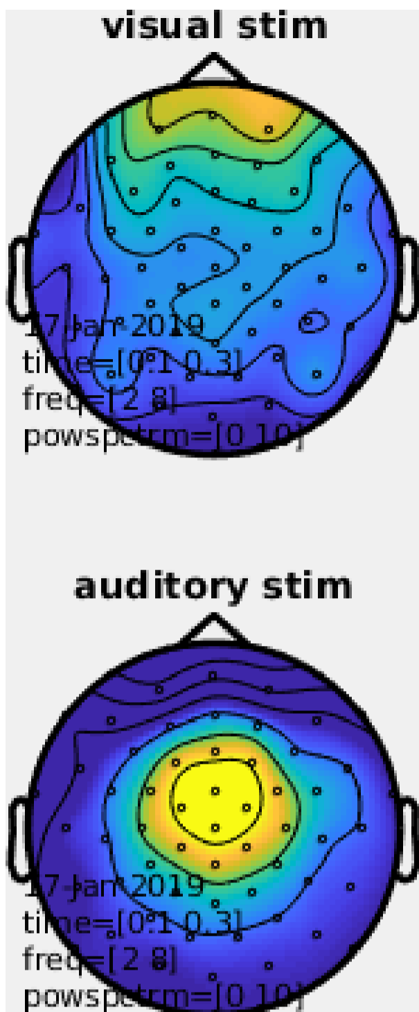
Figure: A topographic representation of the time-frequency representations (3 - 8 Hz, 0.1 - 0.3 s post stimulus) obtained using ft_topoplotTFR
